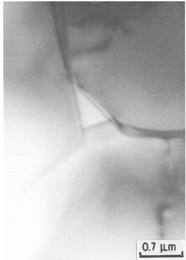
Figure 9 Transmission electron micrograph of mullite ceramics sintered at 1650°C for 4 h showing the glassy phase in a triple junction.
